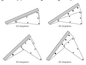
As required, attach the Angle Adjusters to the ends of the keyboard using the 3 screws per end provided (M4 x 12mm pan head Posidrive). Ensure the screws are tight before use. If the Angle Adjusters are not required, replace and tighten the 6 screws into the ends of the Keyboard and keep the Angle Adjusters in the video case ready for use next time.
